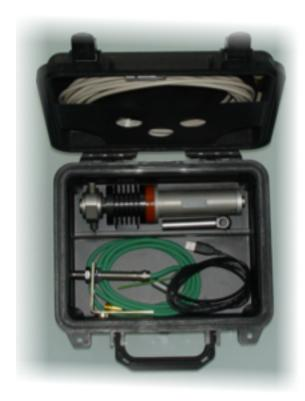
The **Electronic Indicator - EI** is designed by marine engineers to be used from marine engineers. It measures engine performance, monitors the combustion process in diesel engines in real time and allows in-situ engine tuning while measuring. The Electronic Indicator helps balancing cylinder load, optimize injection timing and detect worn or damaged engine components and thus reducing the engine's operating cost.
